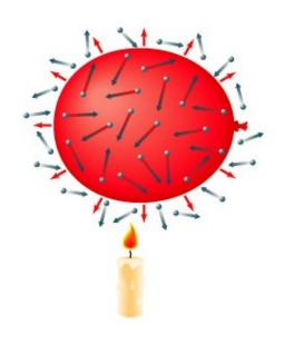
Gas pressure depends on both density and temperature. Adding air molecules increases the pressure in a balloon.
