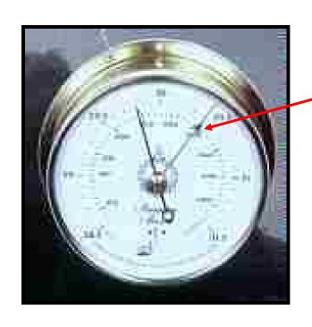
Most aneroid barometers have a needle which can be set to remember the previous reading.
